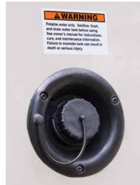
Typical fresh water gravity fill
