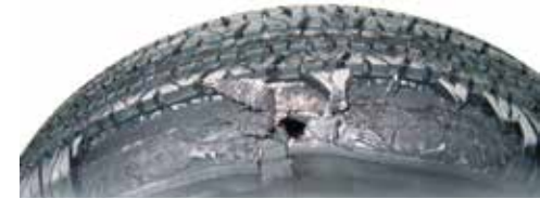
Tire pressure under-inflation can cause serious tire failure
