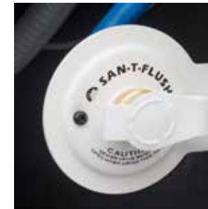
Typical black tank flush
